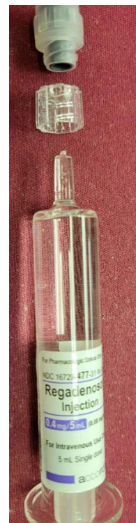
Figure 1. Accord's regadenoson syringe with a protrusion from the tip of the syringe and a disconnected luer syringe connector.
