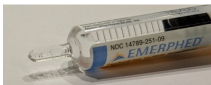
Figure 5. The nurse could not administer medication from the slip-tip connector on the Emerphed (ePHEDrine) glass syringe after the luer connection had come off.
