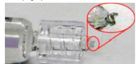
Figure 2. Pin from the LAV connector removed from the syringe tip.
