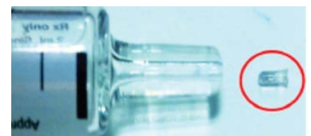
Figure 1. After connecting a glass syringe to the LAV connector, the pin from the connector became clogged in the syringe tip.
