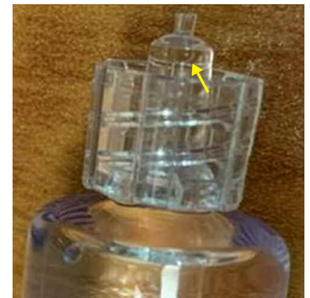
Figure 1. Rather than having an opening at the tip, the syringe is completely sealed with what appears to be a “bubble” of glass (arrow), and the user is unable to expel atropine (Intas Pharmaceuticals) from the syringe.
