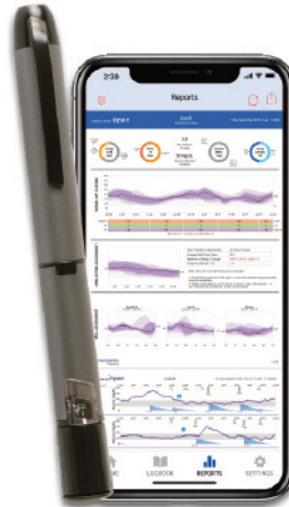
Figure 1. InPen devices are insulin specific and connect with a smart phone app via Bluetooth to help manage diabetes.
