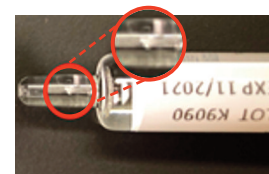
Figure 2. Silicone core appears in nozzle of Dr. Reddy’s naloxone prefilled syringe.
