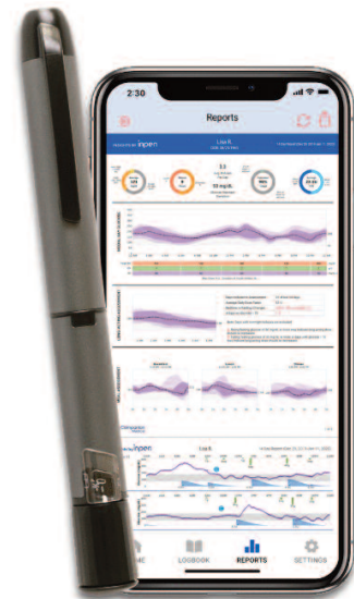
Figure 1. InPen device connects with a smart phone app via Bluetooth to help manage diabetes.
